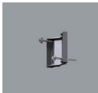
34954.000 Clamping plate for fixing cantilever arm or attachment on upright supporting pole ø 60-89mm. Housing: stainless steel. Graphit m, powder-coated. Cantilever arm or attachment to be ordered separately. Weight 0.80kg Only in conjunction with 34953.000 34955.000
