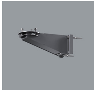
34955.000 Cantilever arm for standing luminaire installation on upright supporting pole ø 60-89mm or wall. Housing: stainless steel. Graphit m, powder-coated. Clamping plate or second cantilever arm for fixing on upright supporting pole to be ordered separately. Upright supporting pole ø 60-89mm to be ordered separately. Weight 2.20kg Only in conjunction with 35718.000
