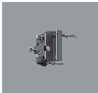
34953.000 Attachment for upright supporting pole ø 60-89mm. Housing: stainless steel. Graphit m, powder-coated. Clamping plate or second attachment for fixing to be ordered separately. Upright supporting pole ø 60-89mm to be ordered separately. Weight 1.00kg Only in conjunction with 35718.000
